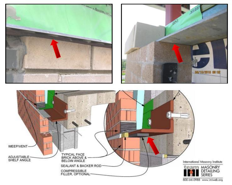
If the masonry is left to be in contact with the metal shelf angle, diagonal cracking at the stress point, bowing of the wall, and corner chipping of the masonry due to point loading will most likely occur.
